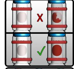
Collect until the appearance of the SVAI changes completely to red. The collection procedure should last approximately 1-5 minutes.
