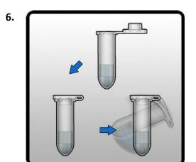
Gently remove the Eppendorf Tubes from the end of the Splitting Unit. Add preservative or stabilising agent for RNA/proteins (not provided), if required, and close the lids on each of the tubes tightly. Invert one of the tubes 2-3 times. Repeat operation for the second tube.
