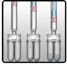
Remove the Collector from the mouth and place the white absorbent pad end into the Compression Tube, holding the Collector in an upright position, and firmly push the plunger downwards to transfer saliva from the absorbent pad into the Collection Tubes. Push and hold for 30 seconds.
