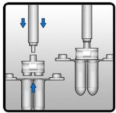
Attach the two Collection Tubes provided to the base of the Splitting Unit. Attach the Compression Tube into the top end of the Splitting Unit firmly. Sample collection may now begin.
